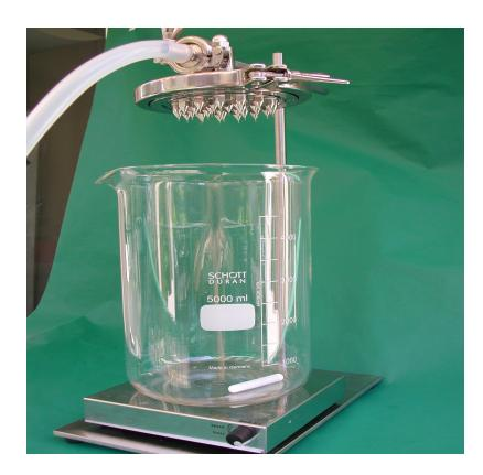
The principle is based on the natural gravity. The liquid goes through the tip of the nozzle, drops grow and separate from the stream (so called normal extrusion in specialist literature), then fall into the hardening solution or goes through another hardening process. Constant permanent flow is used.
